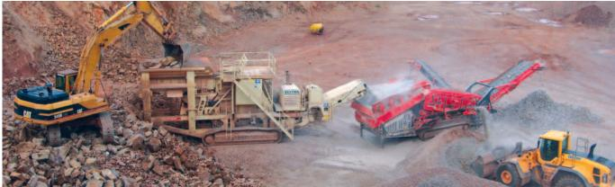
With the largest Contract Crushing fleet in Scotland Leiths have the capability to crush most materials and debris produced in modern construction. Bricks, blocks and concrete can be crushed on site and then re-used on site thus cutting cost and environmental impact, as this mitigates the need to remove material from site and import alternatives.
